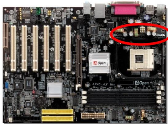
The power circuit of the CPU core voltage must be checked to ensure system stability for high speed CPUs (such as the new Pentium III, or when overclocking). A typical CPU core voltage is 2.0V, so a good design should control voltage between 1.860V and 2.140V. That is, the transient must be below 280mV. Below is a timing diagram captured by a Digital Storage Scope, it shows the voltage transient is only 143mv even when maximum 60A current is applied.
