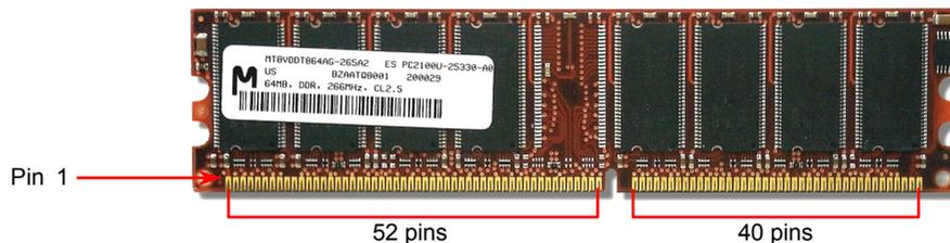
2. Insert the module straight down to the DIMM slot with both hands and press down firmly until the DIMM module is securely in place.
