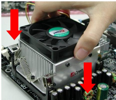
2. Pressing down the four clips with force one by one on the retention module.
