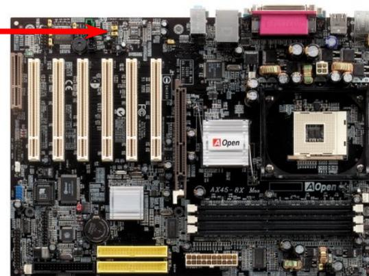
**Note:** Please remove the jumper cap from the front audio connector before you connect the cable. Do not remove this yellow jumper cap if your housing doesn't have an audio port on the front panel.
