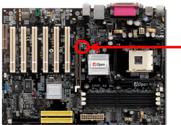
**Warning:** It is strongly recommended not to install a 3.3V AGP card, which is not supported by SIS648. When you do so, the AGP LED on the motherboard will light up to warn you the possible damage.
