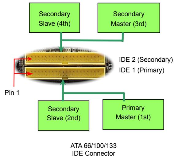
IDE1 is also known as the primary channel and IDE2 as the secondary channel. Each channel supports two IDE devices that make a total of four devices. In order to work together, the two devices on each channel must be set differently to **Master** and **Slave** mode. Either one can be the hard disk or the CDROM. The setting as master or slave mode depends on the jumper on your IDE device, so please refer to your hard disk and CDROM manual accordingly.
