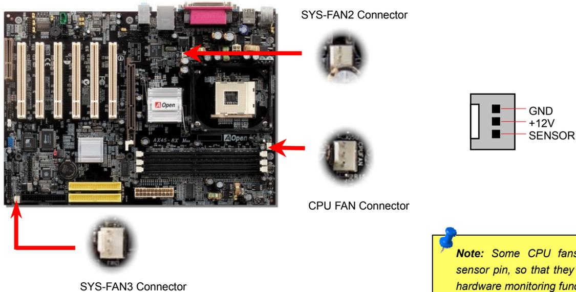
**Note:** Some CPU fans do not have sensor pin, so that they cannot support hardware monitoring function.
